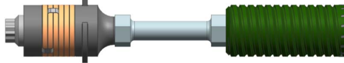
Figure 8 Piezoelectric actuator and coring bit design
